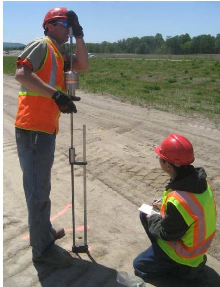
Figure 14. Dynamic cone penetration test
