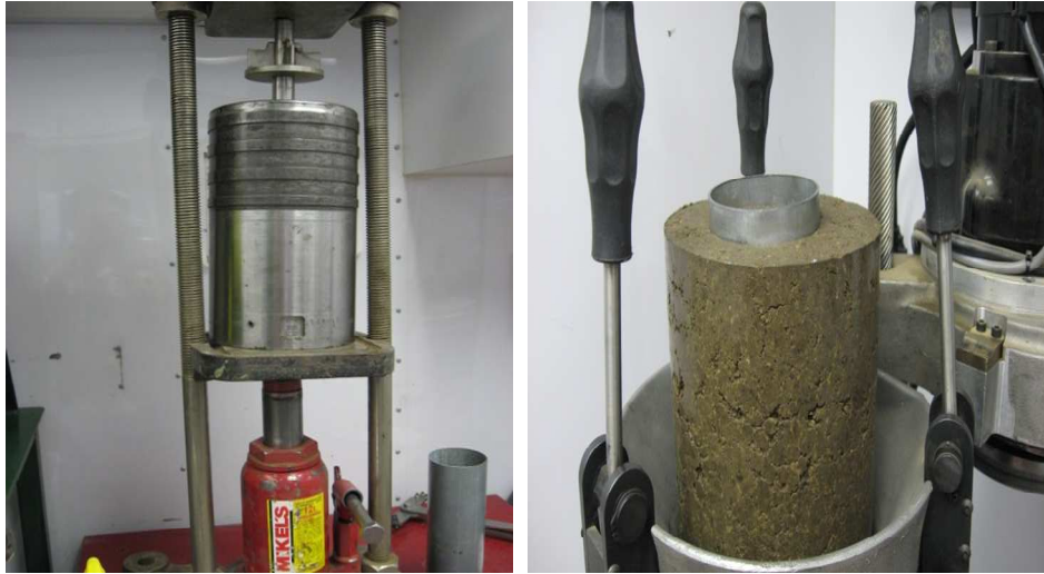
Figure 18. Procedure for inserting Shelby tube into gyratory compacted specimen to generate 2:1 height to diameter ratio specimens
