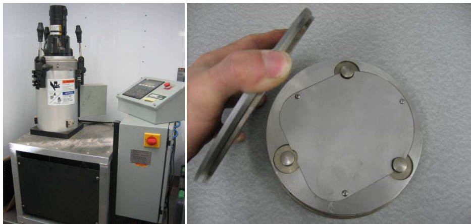
Figure 15. AFGB1A gyratory compactor (left) and pressure distribution analyzer (right)
