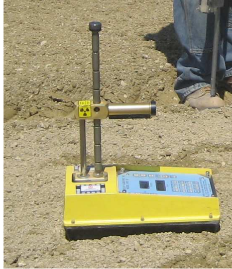
Figure 7. Nuclear moisture-density gauge
