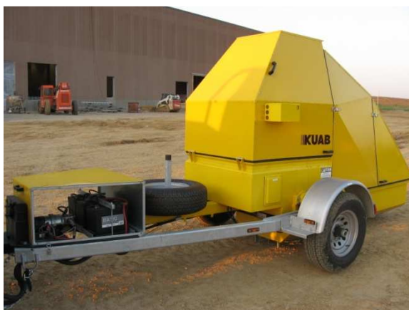
Figure 10. Falling weight deflectometer test with 300-mm diameter plate
