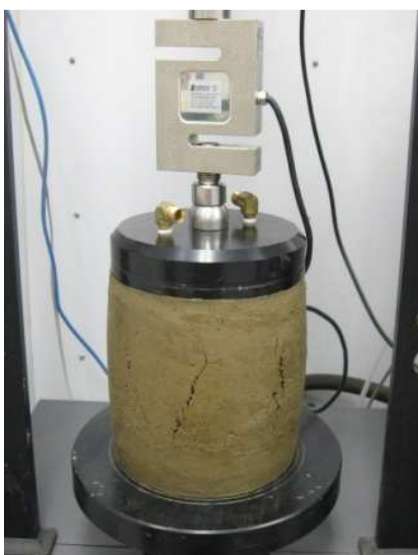
Figure 16. Unconfined compressive test on gyratory compacted specimen
