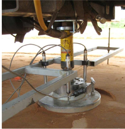
Figure 11. Static plate load test setup with 300-mm diameter plate
